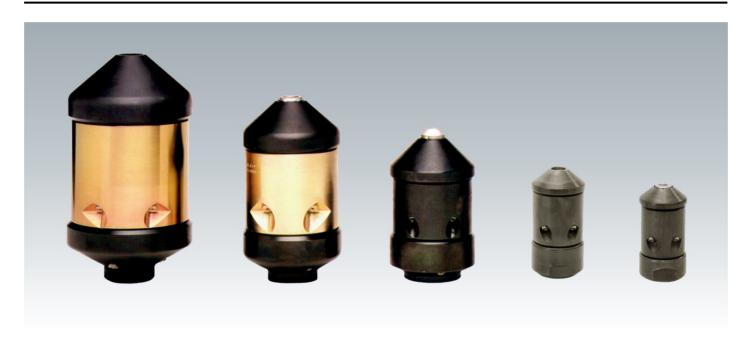
HRH is a nozzle with 4 rotating 45° backward jets. The jets clean the pipe walls and simultaneously they cause a reaction force so that the nozzle is propelled forward.
