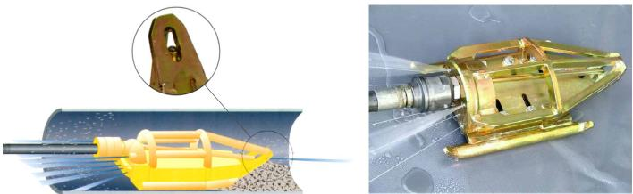
The water jets outs by interchangeable ceramic graft nozzles for long life. It has a configuration so that the water comes outs by the nozzles in laminar flow without turbulence and the jets hit with the maximum effectiveness.
