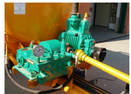
345A Driven by P.T.O. tractor 140 bar - 135 l/min
